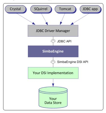
SDK developers create an implementation of a DSI (also known as a DSI Implementation or DSII) that applications use to access the particular data store in the process of executing an SQL statement. In the final executable, the components from SimbaEngine X SDK take responsibility for meeting the data access standards, while the custom DSI implementation takes responsibility for accessing the data store and translating it to the DSI API.
